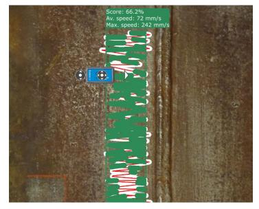
This level of performance also accounts for the beam width, that depends on the UT probe used, and also accounts for the probe skew to make sure you scan with a good orientation.
